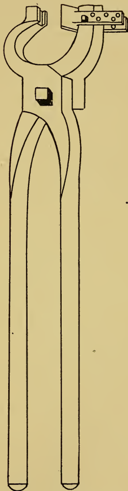
Fig. 4. Adjustable tongs regulated for holding largest size.
